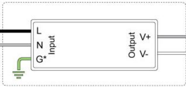
Class 2 Low Voltage Driver*** Installed in Junction Box†
