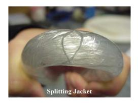
After you score the jacket, you should be able to split it by bending the cable back and forth. Once it's split, run a cut from the split you created toward the end of the cable. You don't have to go far (don't knick and of the fibers inside) before you'll be able to pull the jacket off.
